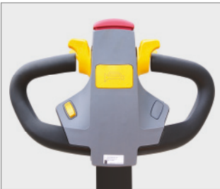
Frei tiller head with one side lifting button (option)
