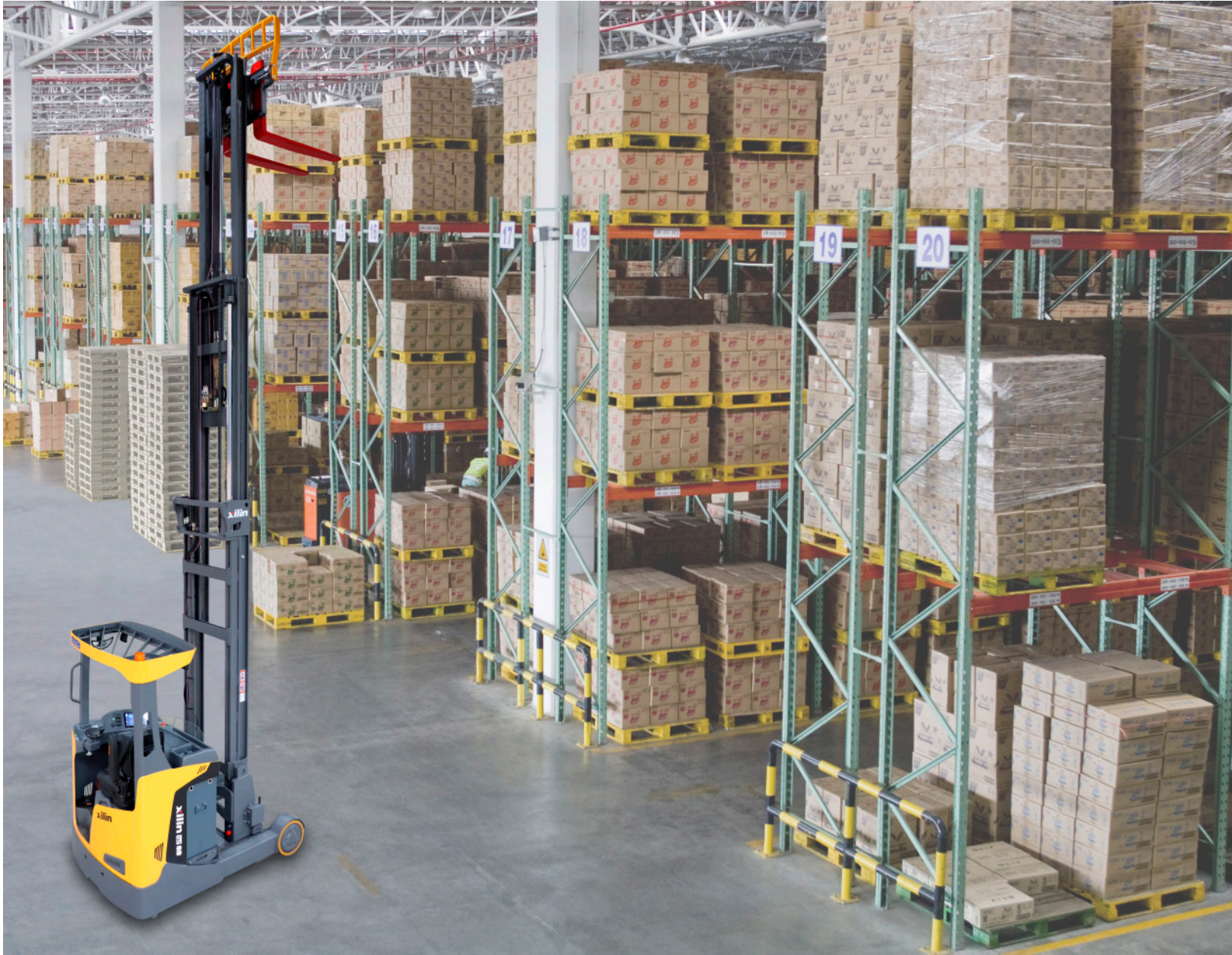
Reach truck with customized mast for Drive-in rack
