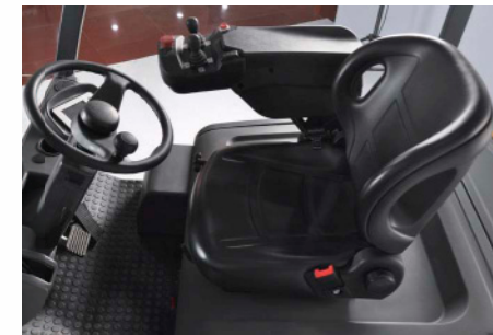
Joystick operation with electro-magnetic valve
